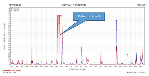
Figure 3-4 Observed versus simulated flows at C3H017.
